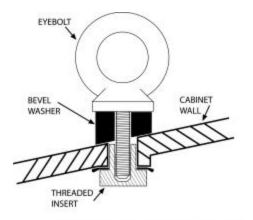
For side inserts, use 6 mm x 1mm pitch x 25.4 mm thread length steel forged shoulder eyebolt.
